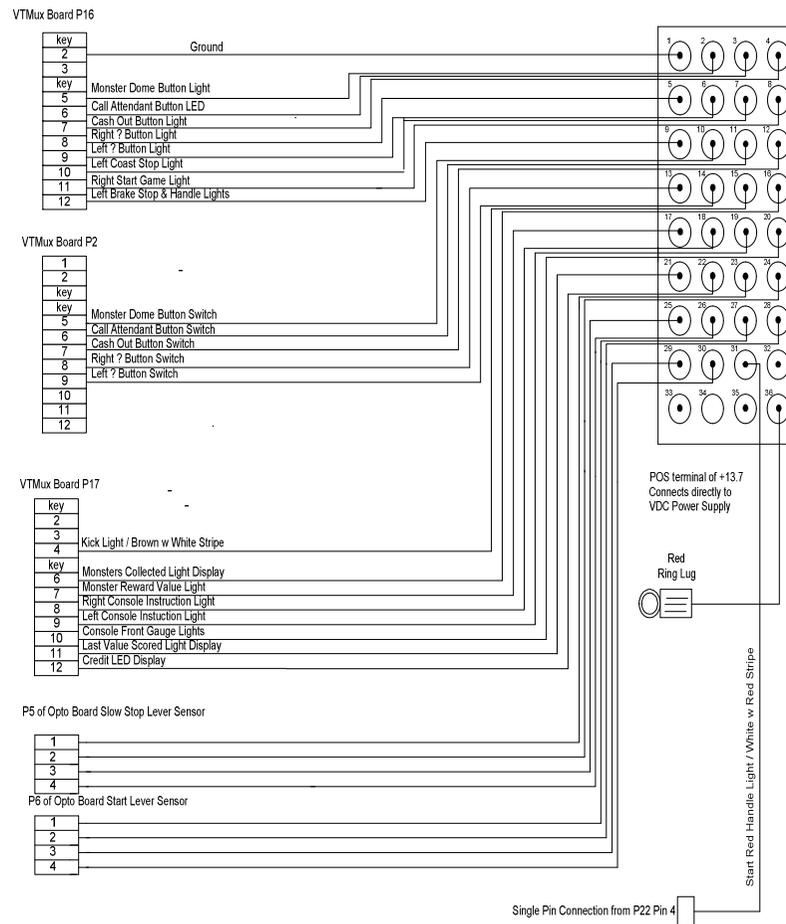
**FIGURE 4 P2, P16, AND P17 CONNECTIONS FROM THE VTMUX BOARD
