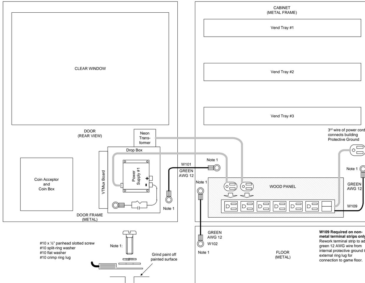
**FIGURE 30 - PROTECTIVE GROUND WIRING**
