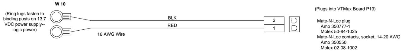
**FIGURE 24 13.7 VDC POWER SUPPLY TO 8051 VTMUX BOARD P19**
