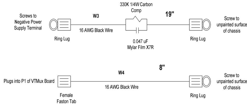
Figure 19 Topper Lights Wiring
