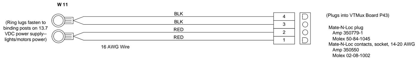
**FIGURE 25 -13.7 VDC POWER SUPPLY TO 8051 VTMUX BOARD P43**
