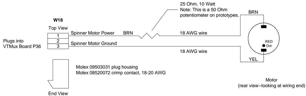
**FIGURE 17 VTMUX BOARD P34 TO SPINNER MOTOR**
