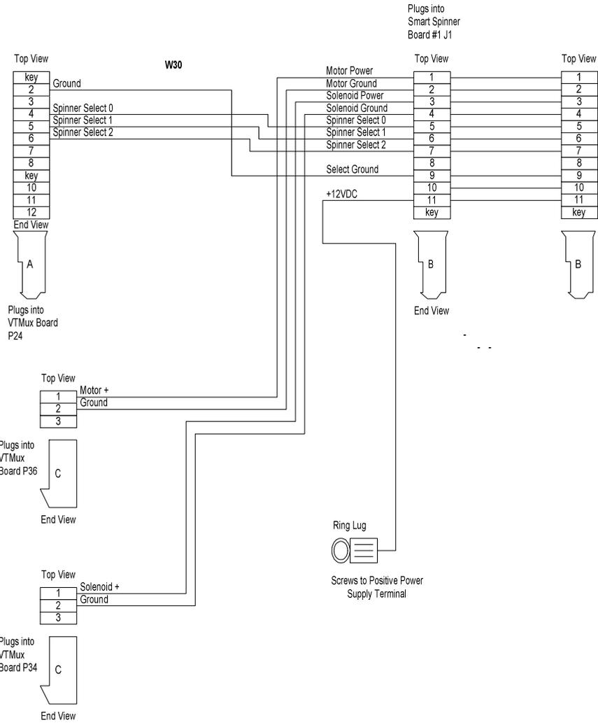
**FIGURE 7 POWER SUPPLY TO SPINNER BOARDS #1 & 2 J1s7
