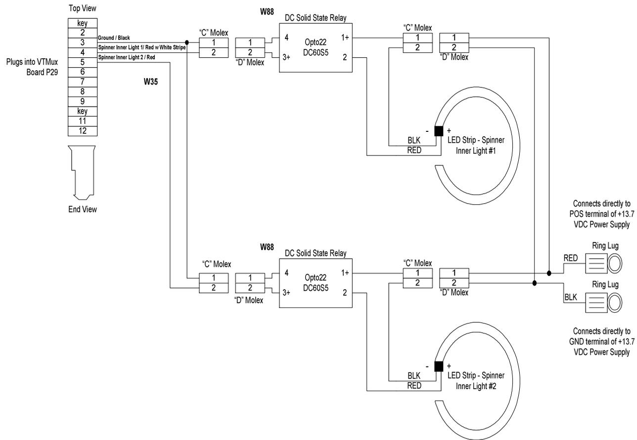
**FIGURE 15 SPINNER'S 1 – 2 NEON RINGS WIRING**
