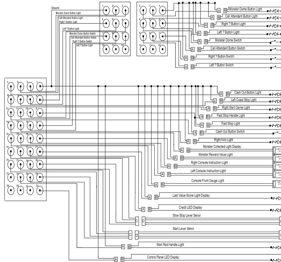
**FIGURE 5 CONNECTIONS TO THE CONTROL PANEL**
