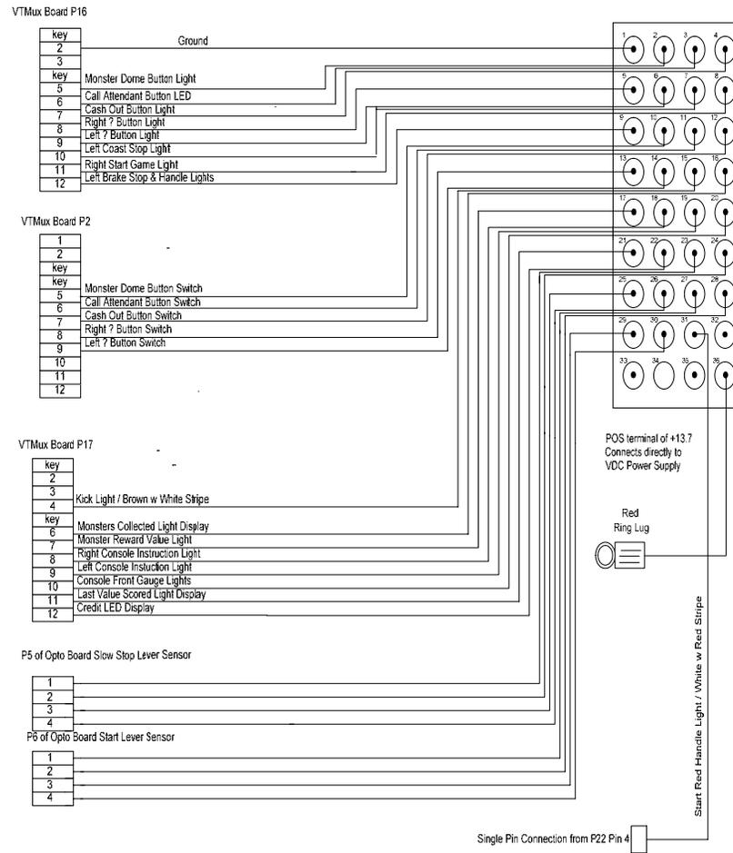
**FIGURE 4 P2, P16, AND P17 CONNECTIONS FROM THE VTMUX BOARD TO THE CONTROL PANEL P5 & P6 FROM OPTO BOARD TO THE CONTROL PANEL**
