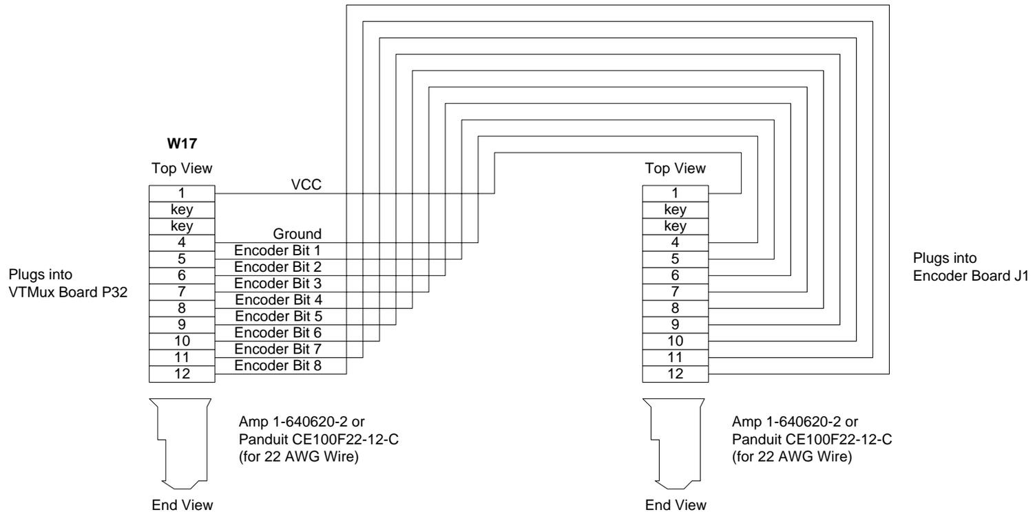
**FIGURE 18 VTMUX BOARD P32 TO SPINNER SHAFT ENCODER**
