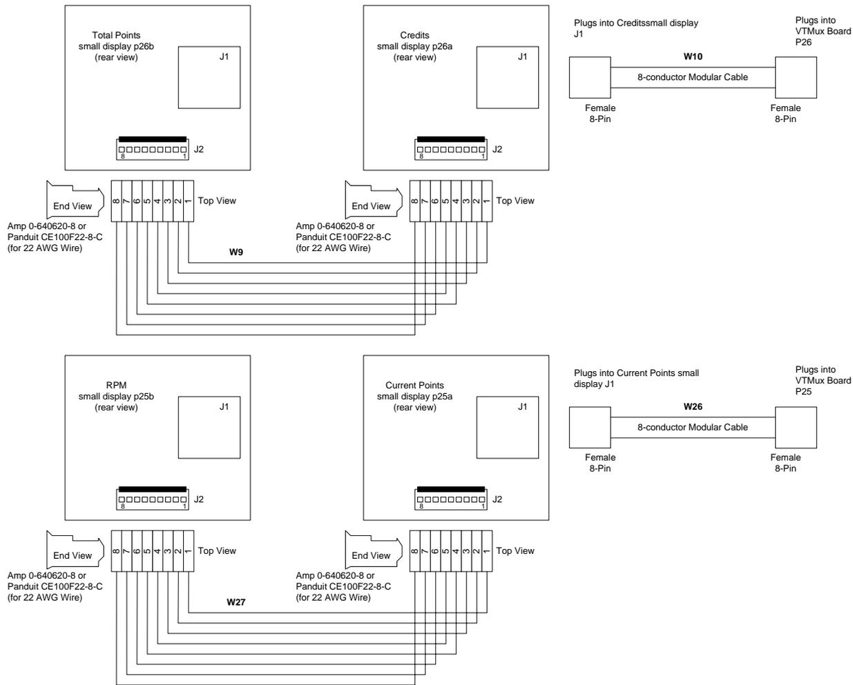
**FIGURE 28A VTMUX BOARD P26 TO CREDITS SMALL DISPLAY J1**
