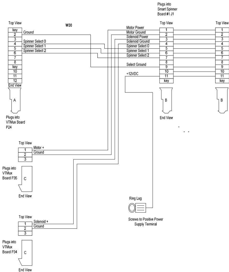
**FIGURE 7 POWER SUPPLY TO SPINNER BOARDS #1 & 2 J1s7
