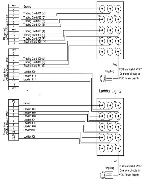
**FIGURE 6 VTMUX BOARD P32 TO SMART SPINNER BOARD #1 & 2, J4s W34**
