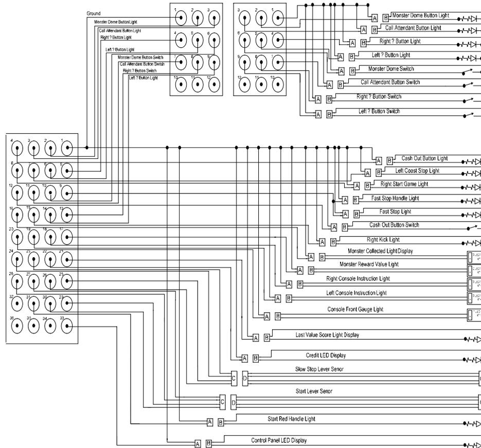
**FIGURE 5 CONNECTIONS TO THE CONTROL PANEL**
