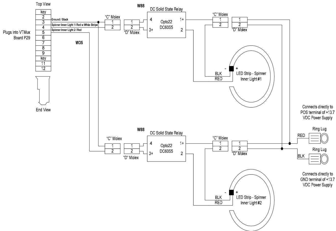
**FIGURE 15 SPINNER'S 1 – 2 NEON RINGS WIRING**
