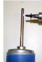
NOTE: UNITS BUILT AFTER 3/01/07 HAVE A NOTCH CUT INTO THE MOTOR SHAFT THAT THE SET SCREW TIGHTENS INTO. IF YOUR UNIT IS DATED AFTER 03/01/07 - THE SET SCREW MUST BE TIGHTENED INTO THIS NOTCH TO FUNCTION.
